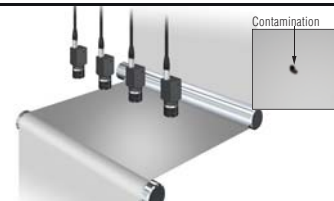
Inspection of pinholes and foreign materials on a sheet
